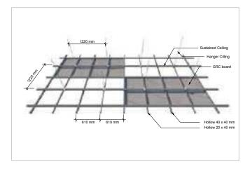
3. Cross Furring system (minimum thickness 0,35 mm).
