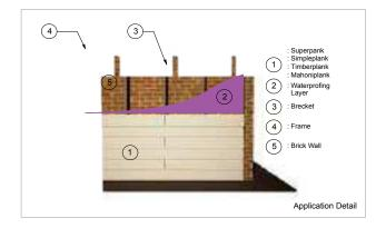
For Finishing on siding plank application could apply water base or oil base paint. Because it is an external application, so it is recommended to apply the paint which is resistant to the weather. To emphasize the colour of the wood for timberplank application, you could apply polish.
