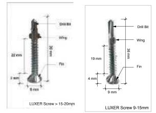
For LUXER Floor application which is sustained by metal framework could apply LUXER Screws for >15 – 20 mm.
