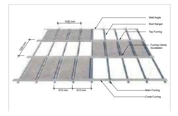
Main tee Cross Frame, for ceiling lay in application. For this application, the board that is usually applied LUXER BOARD which has the dimension 6x600x1200 mm and 6x600x600 mm without drills.
