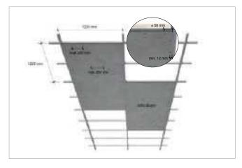
2. LUXER BOARD for Ceiling application is recommende to installed not parallel.
